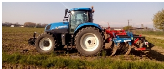
Fig. 1. Tractor and ripper were used in tests.
